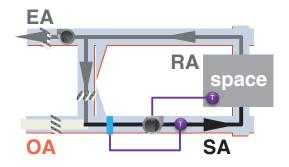
In a Single Zone VAV system, the temperature sensor in the zone is used to vary the air temperature and the air volume in order to maintain the desired set point.
